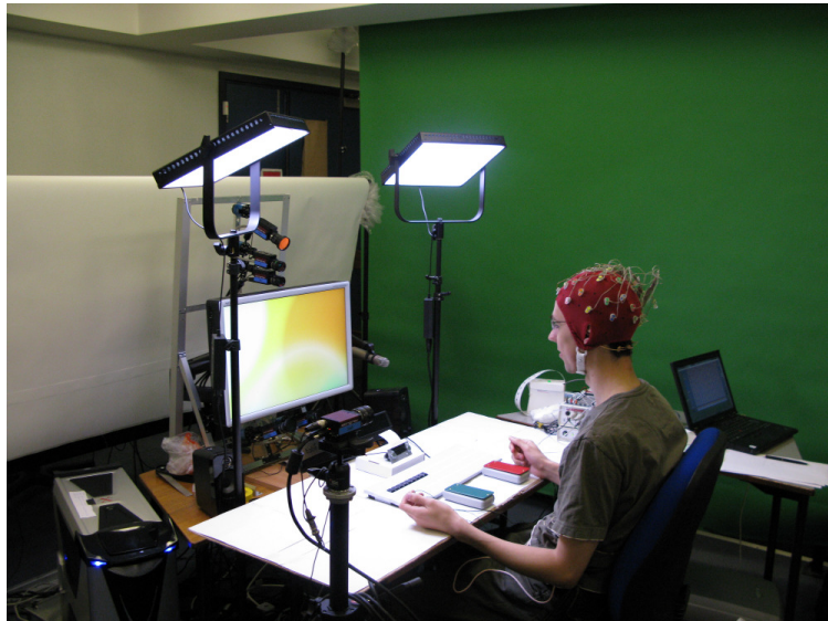
FIGURE 1. In the experimental setup, six video cameras were recording facial expressions. The modified keyboard is visible in front of the participant.
